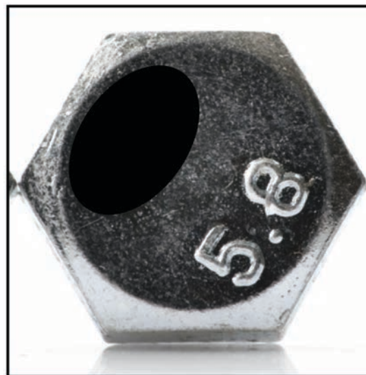
FIGURE 10: EXAMPLE OF ISO 898/1 5.8 HEAD MARKING (BLANK DOT IS MFR. ID)
