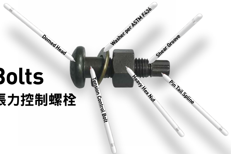
Figure 1: Anatomy of a Tension Control Bolt
