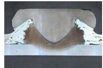
Figure 5: Example of EJOT® EJOWELD® CFF Aluminum to High-Strength Steel Joint
