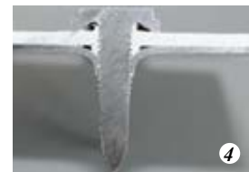
Figure 3: EJOT® FDS® in 3-Layer Stack Figure 4: EJOT® FDS® Aluminum on Steel Stack
