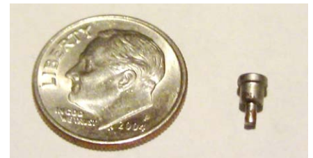
Figure 5: Shoulder Screw for Computer (Blank-Not Threaded Yet)
