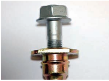
Figure 2: Bolt and Collette Style Caliper Pin
