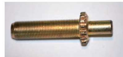
Figure 4: Example of Drum Brake Adjuster Stud
