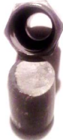
Figure 4: Example of Back Extruded Spark Plug Shell (Leaning on Raw Material Blank)
