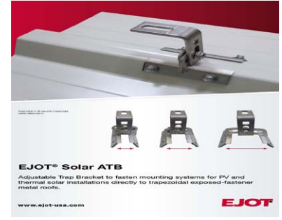
Figure 7 (EJOT® ATB Bracket for Trapezoidal Metal Roof Profile)
