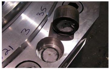
A Socket Head Cap Screw that has Failed by Hydrogen Embrittlement (used with permission of SV Brahimi)
