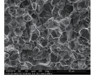
Scanning Electron Microscope Image of a Hydrogen Embrittlement Failure Showing the Characteristic Intergranular Brittle Fracture Morphology (used with permission of SV Brahimi)
