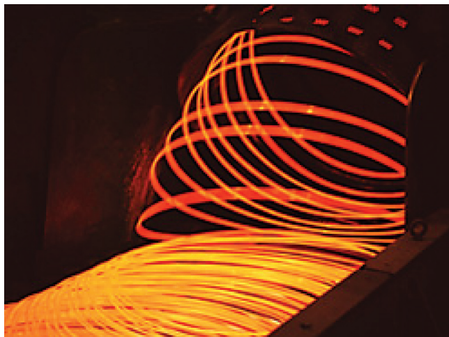
Fig. 3 — Coiled rod exiting the laying head.
