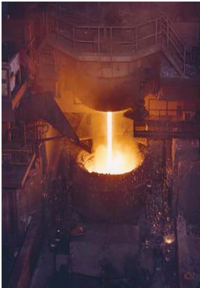
Fig. 2 — Tapping EAF into ladle.
