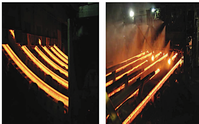
Fig. 4 — Six-strand continuous casting line.
