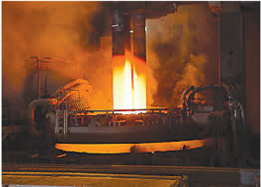
Fig. 1 — An electric arc furnace with electrodes retracted.
