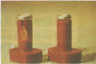
Sheet metal screw DELTA PT® screw 60° flank angle small flank angle
