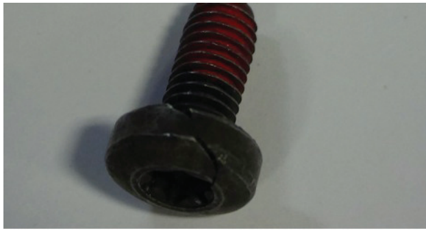
Figure 7: Typical Compression Cracked Head
