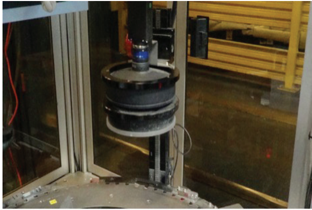
Figure 3: Vertically mounted camera for head cracks
