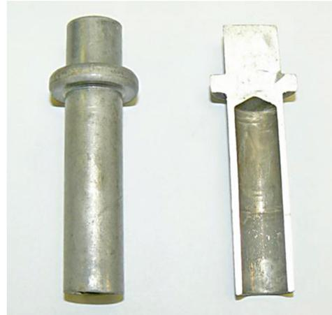
Fig. 2 — External view of the cold formed blank and the internal section.
