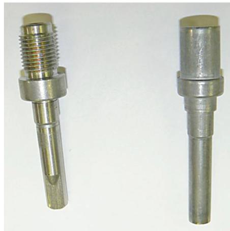
Fig. 3 — Spindle that was originally screw machined.
